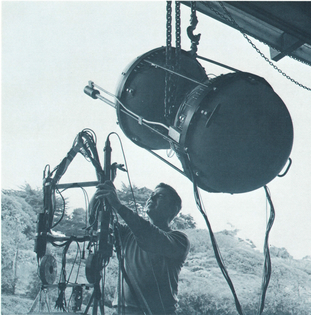
Fig. 2. Temperature sensor assembly is being mounted on an instrument tripod. It can be submerged to depths over 20,000 feet and can make temperature measurements to a resolution of 1/10 millidegree.
